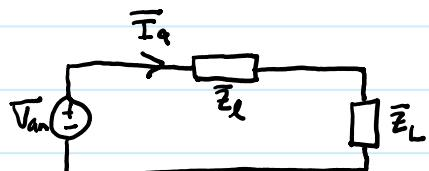
$$\boxed{\overline{I}_a = \frac{\overline{V}_{an}}{\overline{Z}_L + \overline{Z}_L}}$$
