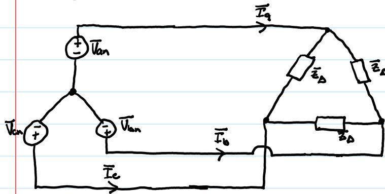
$$\begin{aligned} \bar{V}_{an} &= V_\phi / \Delta \Rightarrow \bar{V}_{ab} = V_\phi \sqrt{3} / 30^\circ \\ \bar{V}_{bc} &= V_\phi \sqrt{3} / -90^\circ \\ \bar{V}_{ca} &= V_\phi \sqrt{3} / 150^\circ \end{aligned} \quad \left. \right\} \text{Wye Rules}$$
