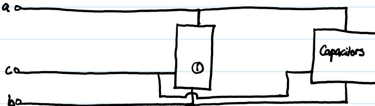
Given:  $P_i = 300 \text{ kW}$        $\text{PF}_i = 0.6 \text{ lag}$
