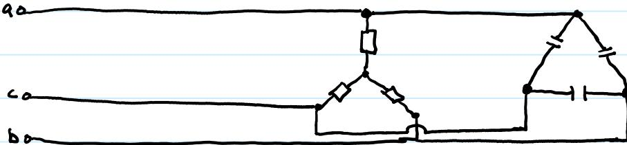
Given:  $V_L = 440 \text{ V}$        $P_{3\phi} = 120 \text{ kW}$        $\text{PF} = 0.85 \text{ lag}$  before adding capacitors
