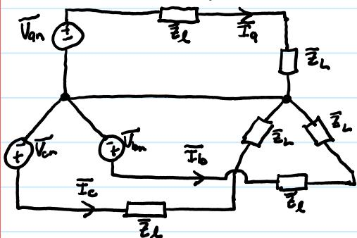
\* We want to calculate  $\overline{I}_a, \overline{I}_b, \overline{I}_c$
