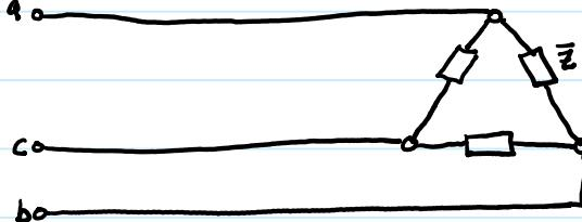
Given:  $V_L = 345 \text{ V}$        $S_{3\phi} = 750 \text{ MVA}$        $\text{PF} = 0.8 \text{ lag}$
