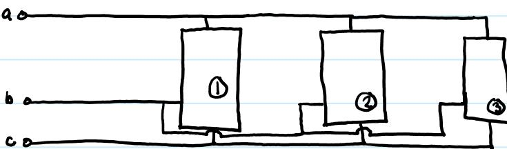
Given:  $V_L = 2400 \text{ V}$ ,       $S_1 = 120 \text{ kVA}$        $\text{PF}_1 = 0.8 \text{ lead}$ ,       $P_2 = 180 \text{ kW}$        $\text{PF}_2 = 0.6 \text{ lag}$ ,       $P_3 = 30 \text{ kW}$        $\text{PF}_3 = 1$
